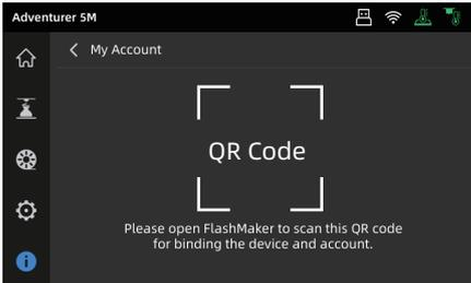
4. Use Flash Maker to scan the QR code on the printer screen to bind the printer to your account.
