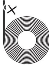
b. Hang the filament on the spool holder. Pass it through the filament sensor until it's seen from the other end of the filament guide tube. Push it forward to the feed roller, until it can not go further. (Please use PLA filament for the first print on initial setup).
