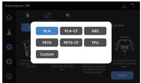
4. Click [Start], wait for the extruder to heat up and filament feeding will begin. When you see the previous filament is extruded, insert the new filament and observe its flow and the extrusion. If the new filament smoothly comes out of the nozzle, the filament change is successful. If not, hold the filament by hand, insert it into the inlet, and click [Again] to retry. Feel for filament movement until it is extruded. After successful loading, insert the filament guide tube into the inlet.
