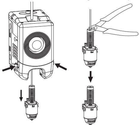
3. Insert the new nozzle into the extruder and you can hear a "click" sound indicating the buckle position has changed. Ensure that the nozzle slot aligns flush with the bottom of the extruder. Note: If you have trouble aligning the nozzle, you can press the buckles during installation or remove the front cover of the extruder (grab the lower part of the front cover with your hand and lift it upward slightly) to check the position.
