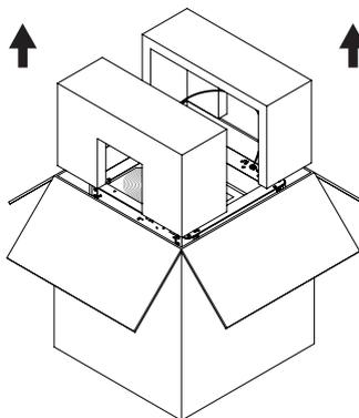
3. Take out the machine, place it on a level workspace and remove the packaging bags and tapes.
