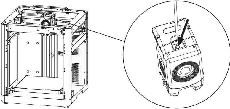
4. Insert the other end of the filament guide tube into the filament detection sensor.
