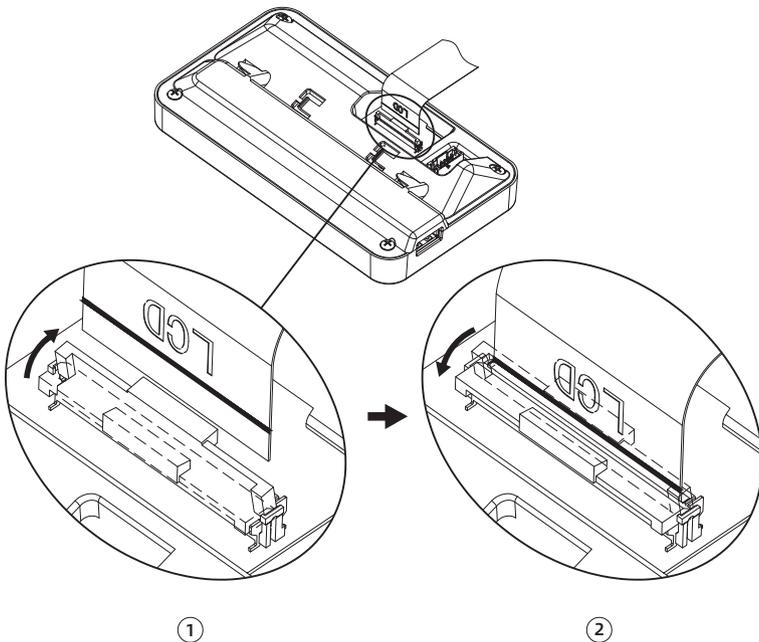
2. Insert the buckle on the back of the screen into the printer's slot, and push the screen according to the arrow direction to lock it in place.
