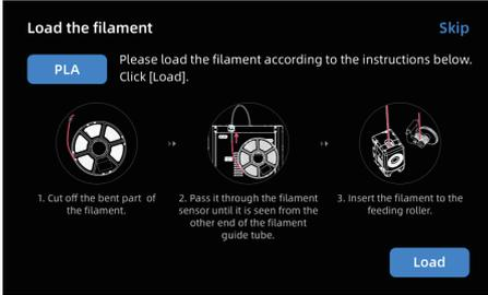
a. Cut off the bent part of the filament end.
