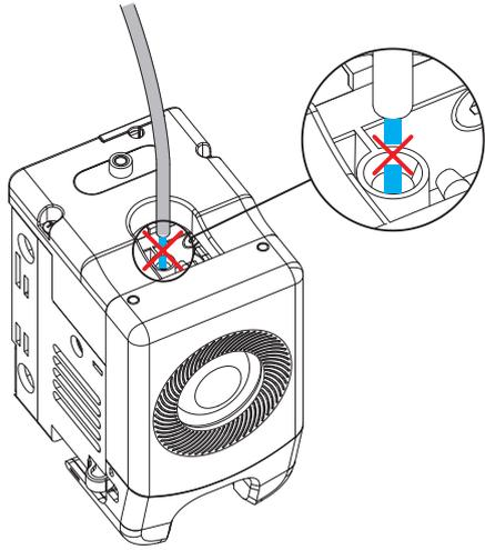
3. Pull out the cut filament, and insert the new filament into the filament guide tube. If the material type is changed, click [PLA] to select the corresponding material type.
