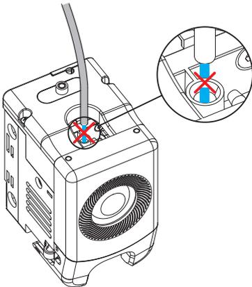
2. Press the left and right buckles and remove the nozzle. Trim the filament along the nozzle top.
