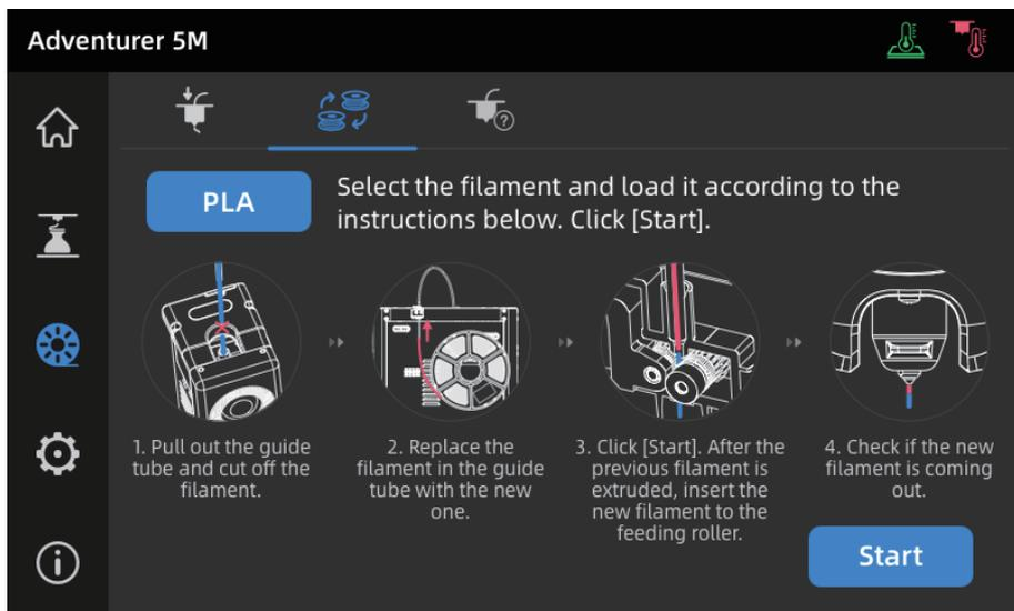
2. Pull out the filament guide tube as shown, and cut the filament.
