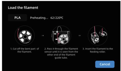
C3. Feeding will begin after heating. Successful filament extrusion from the nozzle indicates successful loading. Lastly, confirm the filament guide tube is properly inserted.
