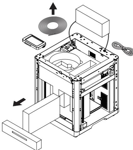
5. Move the chamber foam according to the arrow direction.
